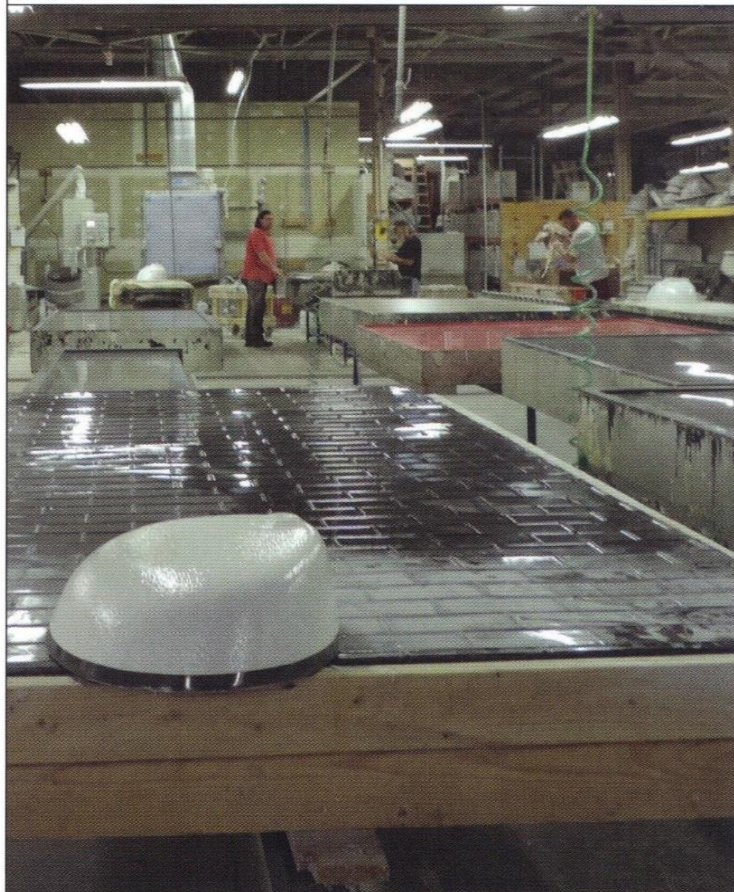
One of Luicana’s newest offerings—subway tile—is made with a special mold that creates a grout-less panel. Above is a finished project. Below is the mold being prepped for pouring.
